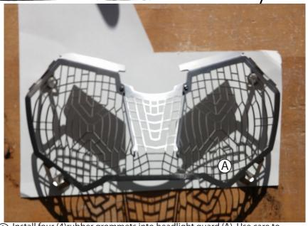
Install four (4) rubber grommets into headlight guard.(A) Use care to not rip the rubber. **!TIP** a dab of water will help them slide into place. Install rubber strip on rear of top edge.(B) Peel protective cover from polycarbonate lens. Install lens as shown with (6) supplied screws, washers, and nuts.(C) Install each screw loose first, then tighten down evenly.
