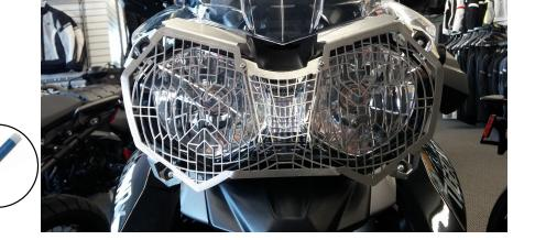
Install headlight guard. **!TIP** A dab of water on each ball stud will help it fit in place easier with less wear on the rubber grommets.
