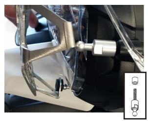
3 Apply a small drop of loctite to the threads of each ball stud. Thread in each upper ball stud on side panels near turn signals. Place one 10mm spacer on remaining ball studs and thread in to holes under front fairing as shown. Tighten to 5Nm
