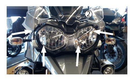
② Use T30 Torx and remove four screws shown. One each just in front of turn signal, and two more under front lower edge of headlight guard (these are at a slight angle).
